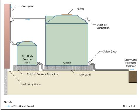
**Roof Washers** are devices placed just before the inflow into the cistern. Roof washers consist of a storage device that allows for some settling, as well as fine screens over the outlet; these devices are intended to treat the fine particulates in runoff. Roof washers must be maintained on a regular basis to prevent clogging. An illustration of one type of roof washer is shown below.
