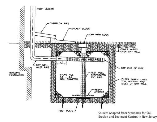
Figure 9.3-1: Dry Well Components
