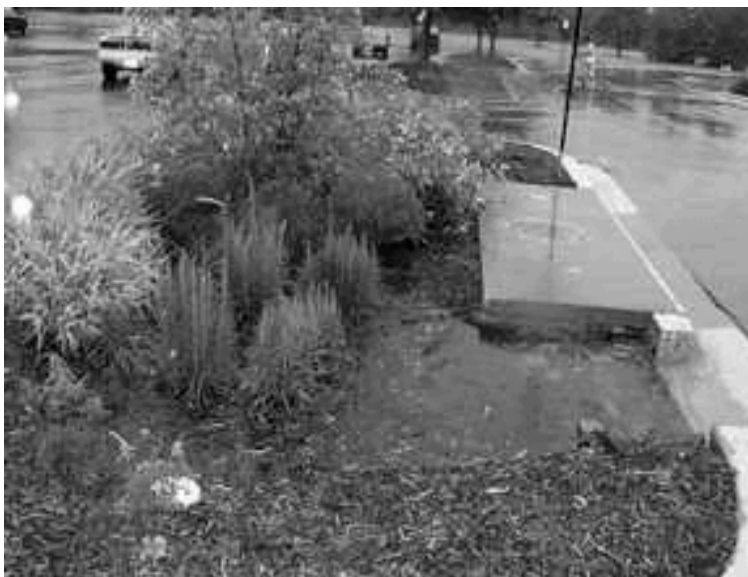
Nonstructural stormwater management strategies include breaking up or disconnecting impervious surfaces.
