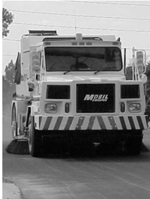
Street sweeping removes solids and floatables from the roadside before they are discharged from the storm drain system.
