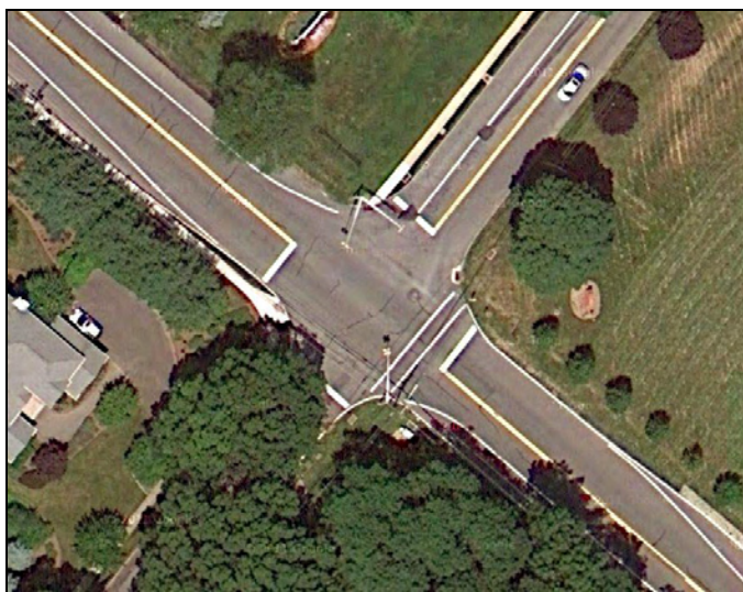
Figure 2-69: Mismatched Crosswalk and Sidewalk at Intersection of NJ 124 and Convent Road
