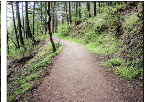
Trail Class 5: Obstacles —Obstacles are not present. Grades are typically less than 8 percent.
